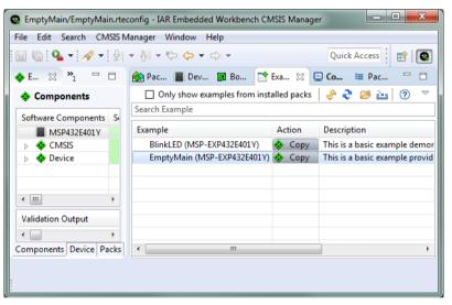
Select an example and click the corresponding action button Copy to copy the CMSIS example project into your IAR Embedded Workbench workspace.
