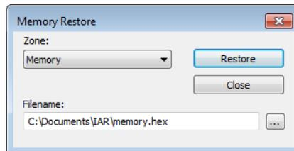
Use this dialog box to load the contents of a file in Intel-extended or Motorola S-record format to a specified memory zone.
