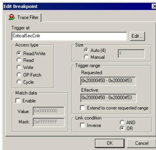
When the trace condition is triggered, the trace data collection is performed for some further instructions, and then the collection is stopped.
