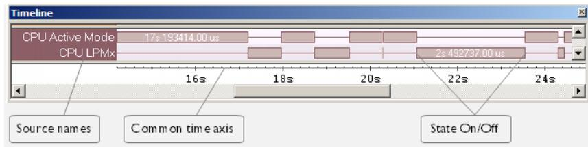
The **State Log** graph displays a graphical view of logged activity—state changes—for peripheral units and clocks, as well as CPU modes in relation to a common time axis.
