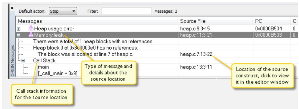
Note that detection of a problem might not occur at the actual point of access. The check might have been moved out of a loop, or several checks for different accesses might have been merged. In these cases, the problem source (the source for the problem access) might not be in the current statement, and there might be more than one problem source.
