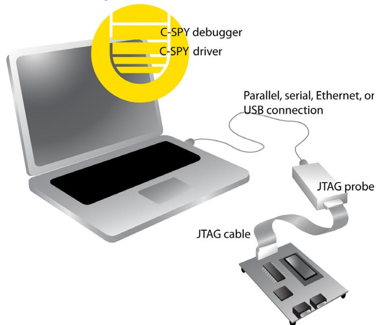
When USB connection is used, a specific USB driver must be installed before you can use the probe over the USB port. You can find the driver on the IAR Embedded Workbench for Arm installation media.
