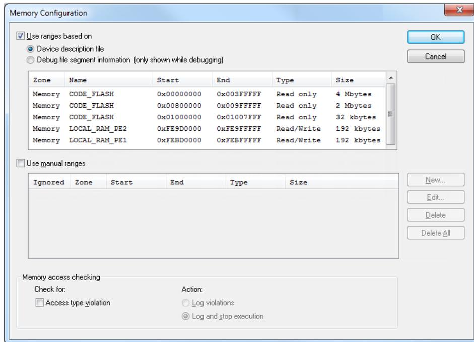
Use this dialog box to specify which set of memory address ranges to be used by C-SPY during debugging.
