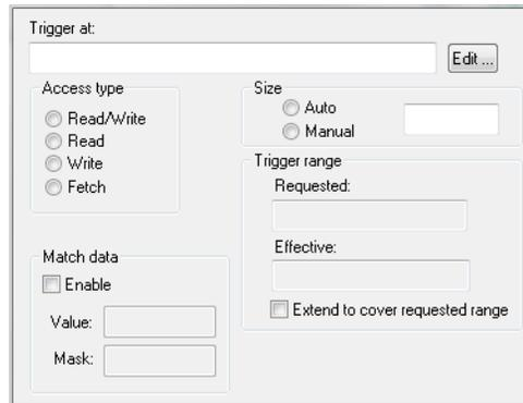
Use this dialog box to set the conditions that determine when to start collecting trace data. When the trace condition is triggered, the trace data collection is started.
