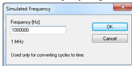
Use this dialog box to specify the simulator frequency used when the simulator displays time information.
