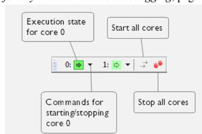
This toolbar is a complement to and shows the same state as the **Cores** window. Each core has a button with an adjacent drop-down menu. Click a button to make C-SPY focus on that core.
