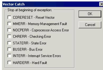
Use this dialog box to set a breakpoint directly on a vector in the interrupt vector table, without using a hardware breakpoint. You can set breakpoints on vectors for Arm9/10/11 and all Cortex devices. Note that the settings you make here will not be preserved between debug sessions.
