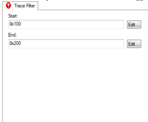
Use this dialog box to set the conditions that determine when to start collecting trace data. When the trace condition is triggered, the trace data collection is started.
