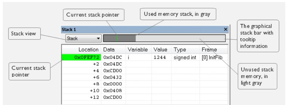
This window is a memory window that displays the contents of the stack. The graphical stack bar shows stack usage.
