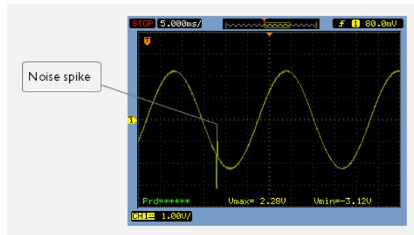
Power debugging will help you investigate interference from digital and power supply lines into the analog parts. Power spikes in the vicinity of AD conversions could be the source of noise and should be investigated. All data presented in the **Timeline** window is correlated to the executed code. Simply double-clicking on a suspicious power value will bring up the corresponding C source code.
