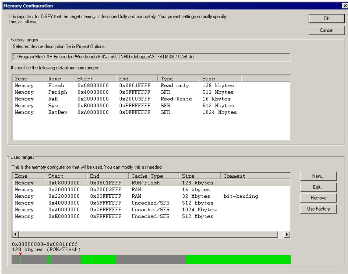
C-SPY uses a default memory configuration based on information retrieved from the device description file that you select, or if memory configuration is missing in the device description file, tries to provide a usable factory default. See *Selecting a device description file*, page 53.
