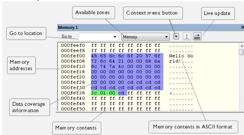
This window gives an up-to-date display of a specified area of memory—a memory zone—and allows you to edit it. You can open several instances of this window, which is very convenient if you want to keep track of several memory or register zones, or monitor different parts of the memory.
