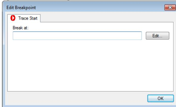
Use this dialog box to set a Trace Start breakpoint where you want to start collecting trace data. If you want to collect trace data only for a specific range, you must also set a Trace Stop breakpoint where you want to stop collecting data.
