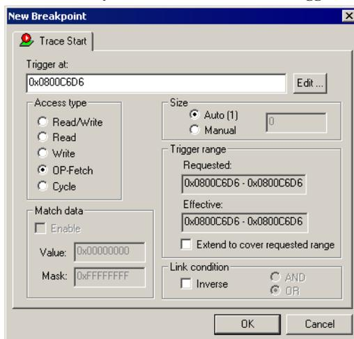
Use this dialog box to set the conditions that determine when to start collecting trace data. When the trace condition is triggered, the trace data collection is started.
