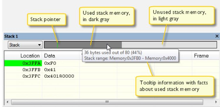
**Note:** Although this is a reasonably reliable way to track stack usage, there is no guarantee that a stack overflow is detected. For example, a stack *can* incorrectly grow outside its bounds, and even modify memory outside the stack area, without actually modifying any of the bytes near the end of the stack range. Likewise, your application might modify memory within the stack area by mistake.
