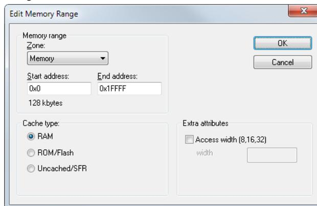
Use this dialog box to specify the memory address ranges, and assign a cache type to each range.
