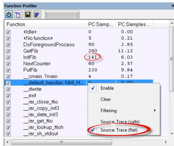
To secure valid data when using a debug probe, make sure to use the maximum trace buffer size and set a breakpoint in your code to stop the execution before the buffer is full.
