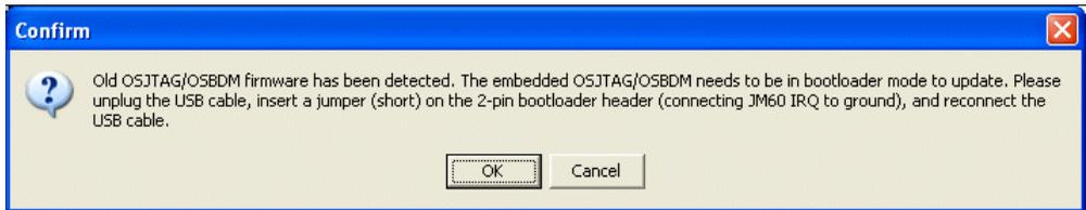
The user should unplug the Tower card from the PC and place a jumper on the 2-pin "JM60 Boot" header. For example, on the TWR-K40X256 board or the TWR-K60N512 board, a jumper should be placed on header J21. When the unit is plugged back into the PC, the user may need to wait for the drivers to properly install before continuing (first time update only). Once the driver installation is complete, or if the driver installation wizard does not appear, click OK.
