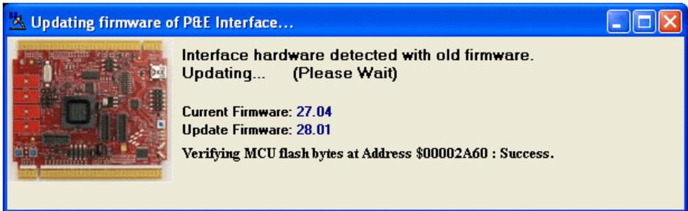
The user is then prompted to remove the jumper. Remove the jumper, unplug the Tower card from the PC, and then plug it back into the PC. Once this is done, click the Ok button to continue with the debug session. You will only need to update the firmware once.
