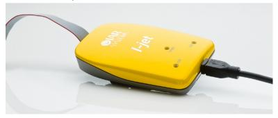
I-jet streams the program counter, variables, and power measurement data to the host computer to provide a view into program execution in real time. Besides the typical JTAG debugging, I-jet is capable of providing power to the target board and measuring
