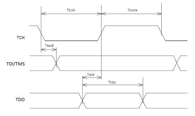
In a JTAG device that fully complies to IEEE1149.1 standard, the TDI/TMS signals should be sampled on the rising edge of TCK, and TDO should be sent on the falling edge of TCK. I-jet takes advantage of these requirements and changes its TDI and TMS signals on the falling edge of TCK and samples the TDO on the rising edge of TCK. However, to accommodate target boards with long JTAG chains and fast JTAG clocks, I-jet allows TDO to be as late as 50 ns after the rising edge of TCK.
