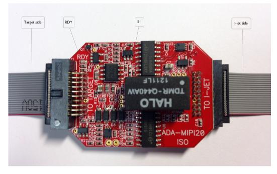
The adapter is automatically recognized by the C-SPY, and the adapter powers up and the green **RDY** LED is turned on.
