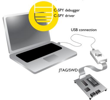
I-jet communicates using USB 2.0. USB 1.0 is also supported but not advised. The I-jet in-circuit debugging probe is also referred to as a debug probe, debug adapter, or JTAG in-circuit emulator by different tool vendors.
