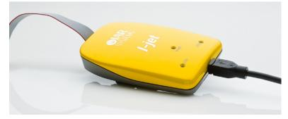
I-jet streams the program counter, variables, and power measurement data to the host
