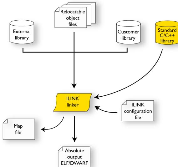
During the linking, ILINK might produce error messages and logging messages on `stdout` and `stderr`. The log messages are useful for understanding why an application was linked as it was. For example, why a module or section (or section fragment) was included.
