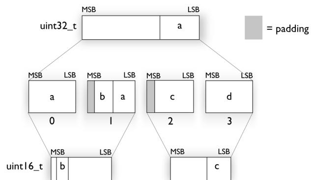
In big-endian mode, each bitfield is allocated starting from the most significant free bit of its container to ensure that it is placed into bytes from left to right.
