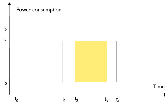
Figure 102: Power consumption in an event-driven system
