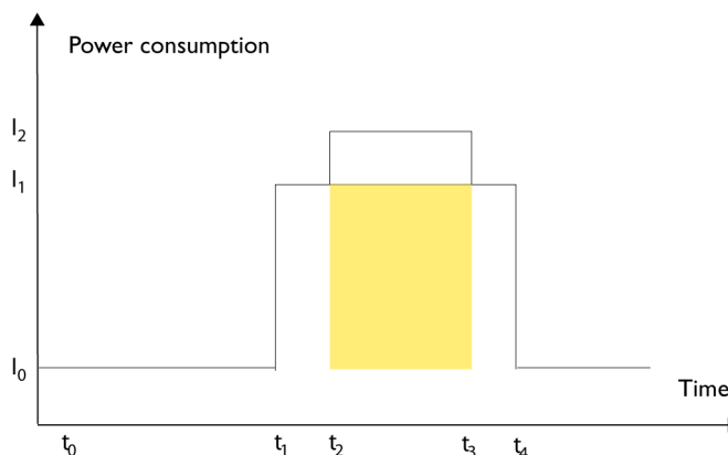
Figure 97: Power consumption in an event-driven system
