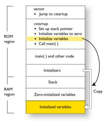
Then, dynamically initialized static objects are constructed, such as C++ objects.
