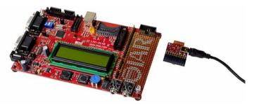
**IAR J-Link** is a JTAG hardware debug probe which connects via USB to the host PC. **IAR J-Trace** is a high-speed hardware trace probe that also connects via USB to the host PC.
