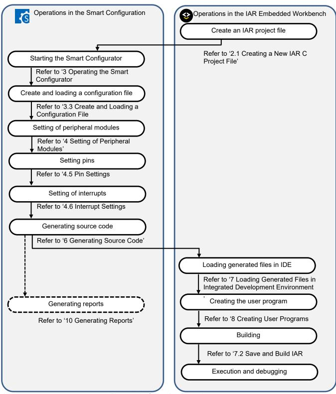
Figure 3-1. Operating Procedure
