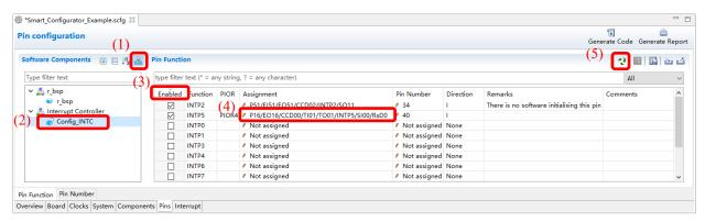
Figure 4-44 Pin Settings - Assigning Pins on the [Pin Function] List
