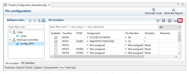
Figure 4-47. Importing Pin Settings from an XML File
