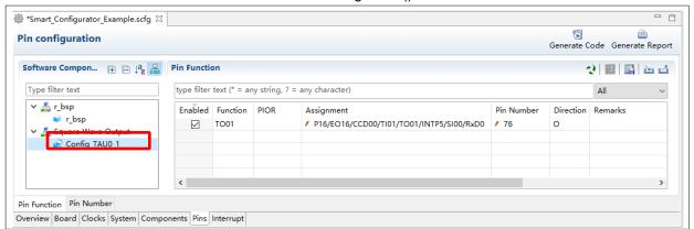
Figure 6-3. Config\_TAU0\_1 in Software Components View
