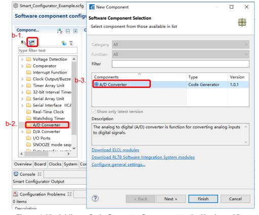
Figure 4-15. Adding a Code Generator Component to the Hardware View
