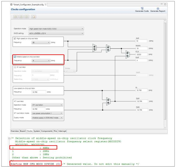
Figure 6-2. Clocks Configuration and Generated Code in r\_bsp\_config.h
