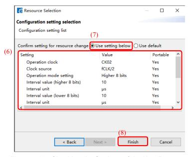
Figure 4-20. Checking the Settings of the New Resource
