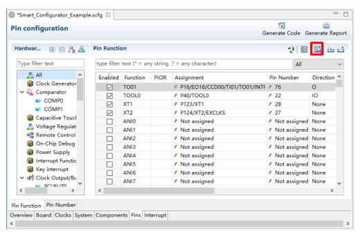
Figure 10-3. Output of a List of Pin Functions or Numbers (in csv Format)
