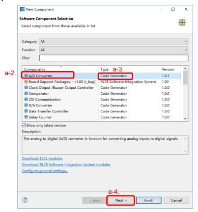
Figure 4-13. Adding a Code Generator Component
