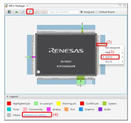
Figure 4-45. Assigning Pins Using the MCU Package View
