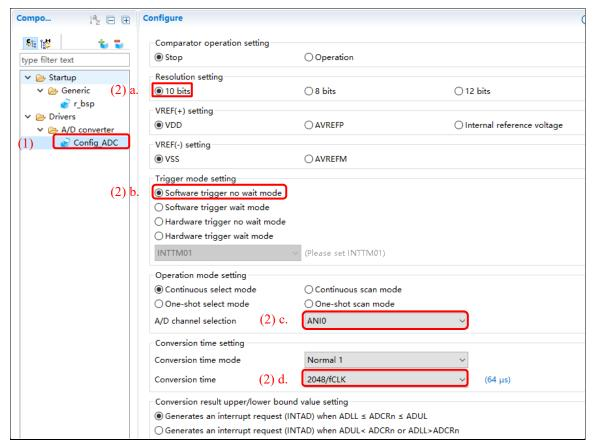
Figure 4-17. Setting of a Code Generator Driver
