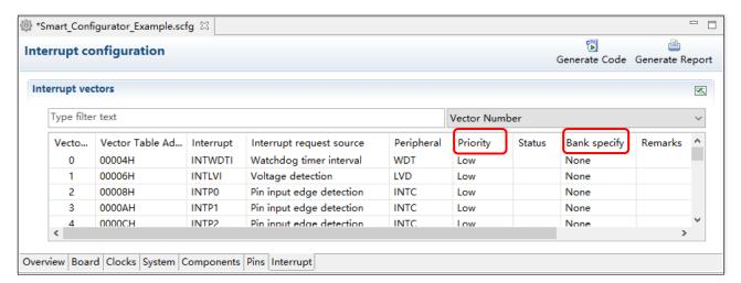
Figure 6-7. Interrupts Configuration in Interrupts View
