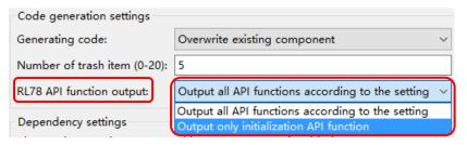
Figure 4-38. [RL78 API function output] Change
