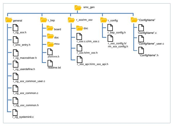
Figure 6-2. Configuration of Generated Files and File Names
