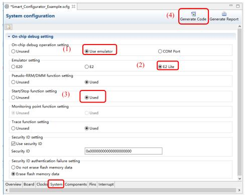
Figure 4-8. Smart Configurator [System] Page Setting
