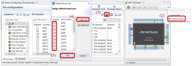
Figure 4-48. Setting for Initial Pin Configuration
