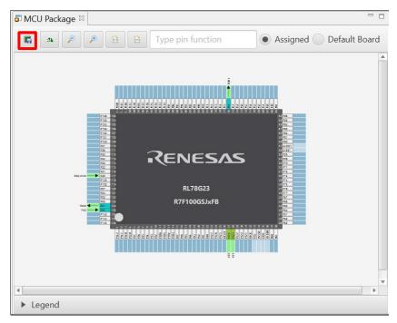
Figure 10-4. Outputting a Figure of MCU Package (in png Format)
