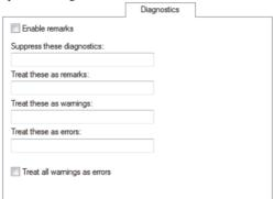
**Note:** The diagnostic messages cannot be suppressed for fatal errors, and fatal errors cannot be reclassified.
