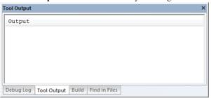
This window displays any messages output by user-defined tools in the **Tools** menu, provided that you have selected the **Redirect to Output Window** option in the **Configure Tools** dialog box, see *Configure Tools dialog box*, page 82. When opened, this window is, by default, grouped together with the other message windows.
