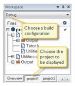
For each file that has been built, an Output folder icon appears, containing generated files, such as object files and list files. The latter is only generated if the list file option is enabled. The Output folder related to the project node contains generated files related to the whole project, such as the executable file and the linker map file (if the list file option is enabled).
