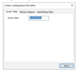
Use this dialog box to specify memory locations for linker sections and blocks in the linker configuration file.
