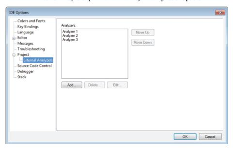
Use this page to add an external analyzer to the standard build toolchain. External analyzers operate on C/C++ source code in the user project. Header files or assembler source code files are not analyzed.
