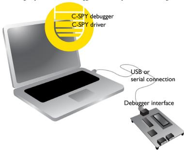
Other target systems have all debugger functionality located on the target board itself:
