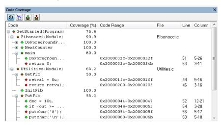
This window reports the status of the current code coverage analysis. For every program, module, and function, the analysis shows the percentage of code that has been executed since code coverage was turned on up to the point where the application has stopped. In addition, all statements that have not been executed are listed. The analysis will continue until turned off.
