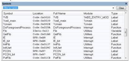
This window displays all symbols with a static location, that is, C/C++ functions, assembler labels, and variables with static storage duration, including symbols from the runtime library.
