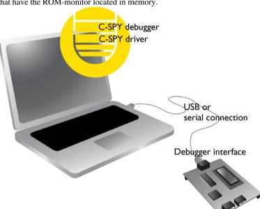
Using the C-SPY ROM-monitor driver, C-SPY can connect to various target hardware that have the ROM-monitor located in memory.
