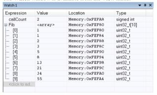
Use this window to monitor the values of C-SPY expressions or variables. You can open up to four instances of this window, where you can view, add, modify, and remove expressions. Tree structures of arrays, structs, and unions are expandable, which means that you can study each item of these.
