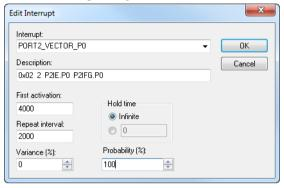
Use this dialog box to interactively fine-tune the interrupt parameters. You can add the parameters and quickly test that the interrupt is generated according to your needs.
