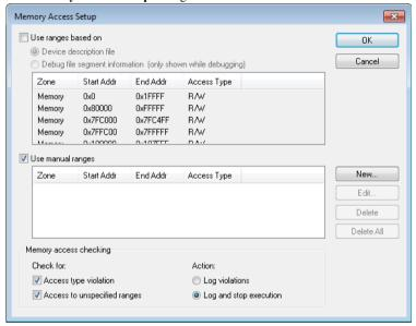
Use this dialog box to specify which set of memory address ranges to be used by C-SPY during debugging.
