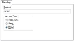
Use the **Data Log** breakpoints dialog box to set a maximum of four data log breakpoints on memory addresses, see *Setting breakpoints using the dialog box*, page 112.
