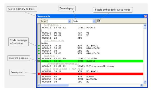
This window shows the application being debugged as disassembled application code.
