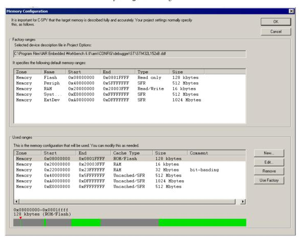
C-SPY uses a default memory configuration based on information retrieved from the device description file that you select, or if memory configuration is missing in the device description file, tries to provide a usable factory default. See *Selecting a device description file*, page 45.
