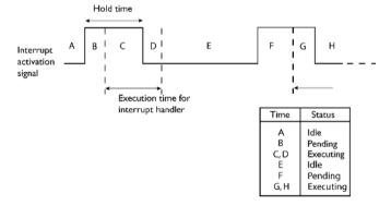
However, if the interrupt repeat interval is shorter than the execution time, and the interrupt is reentrant (or non-maskable), the status information at different times looks like this:
