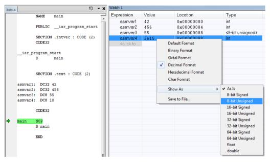
Note that asmvar4 is displayed as an int, although the original assembler declaration probably intended for it to be a single byte quantity. From the context menu you can make C-SPY display the variable as, for example, an 8-bit unsigned variable. This has already been specified for the asmvar3 variable.
