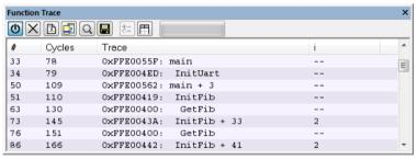
This window displays a subset of the trace data displayed in the **Trace** window. Instead of displaying all rows, the **Function Trace** window shows:
