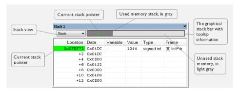
This window is a memory window that displays the contents of the stack. The graphical stack bar shows stack usage.
