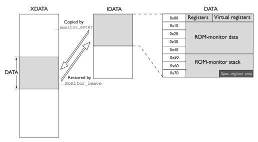
All memory except for the range  $0 \times 78-0 \times 7F$  is restored when switching between the ROM-monitor and the application program.
