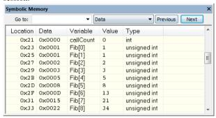
This window displays how variables with static storage duration, typically variables with file scope but also static variables in functions and classes, are laid out in memory. This can be useful for better understanding memory usage or for investigating problems caused by variables being overwritten, for example buffer overruns. Other areas of use are spotting alignment holes or for understanding problems caused by buffers being overwritten.
