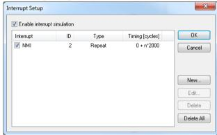
This dialog box lists all defined interrupts. Use this dialog box to enable or disable the interrupt simulation system, as well as to enable or disable individual interrupts.
