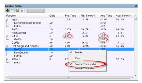
The second figure shows the result of profiling using **Source: Trace (flat)**. In this case, the profiler does not follow the program flow, instead the profiler only detects whether the PC address is within the function scope. For incomplete trace data, the data might contain minor errors.
