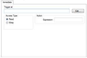
In the C-SPY simulator, you can use the **Immediate** breakpoints dialog box to set an immediate breakpoint, see *Setting breakpoints using the dialog box*, page 112. Immediate breakpoints do not stop execution at all; they only suspend it temporarily.
