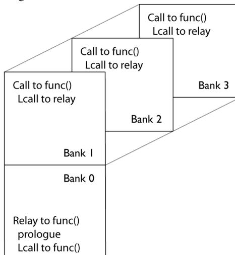
When the callee function has executed, it performs an `?LCALL` to `?BRET`. In `?BRET`, the bank number of the caller function is popped from the `idata` stack and then a `RET` instruction is executed. The execution is now back in the caller function.
