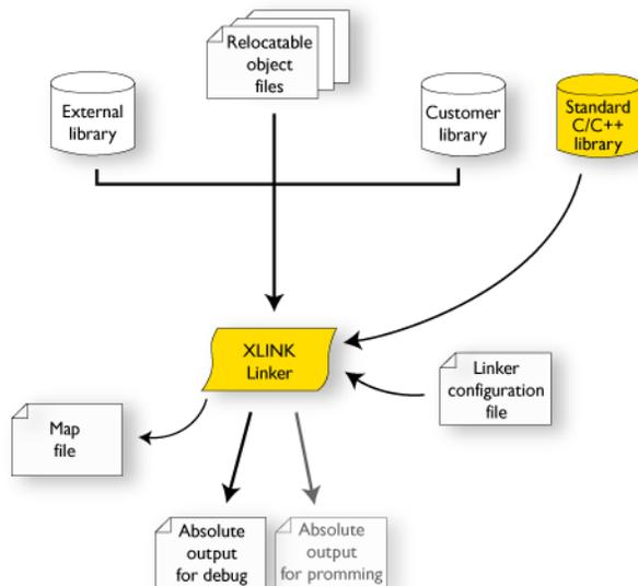
During the linking, XLINK might produce error messages and optionally a map file. In the map file you can see the result of the actual linking and is useful for understanding why an application was linked the way it was, for example, why a segment part was included. If a segment part is not included although you expect it to be, the reason is *always* that the segment part was not referenced to from an included part.
