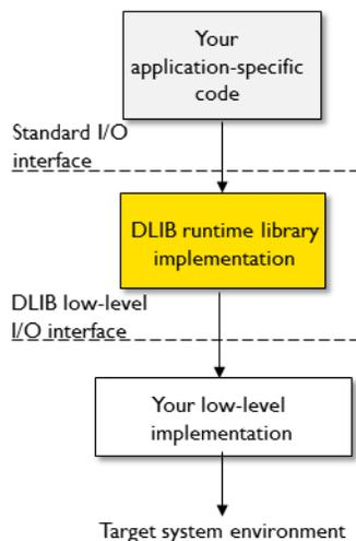
For example, if your application calls the functions `printf` and `fputc` in the standard I/O interface, the implementations of those functions both call the low-level function `__write` to output individual characters. To make them work, you just need to provide an implementation of the `__write` function—either by implementing it yourself, or by using a third-party implementation.
