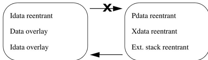
The arrow means that a call is possible. The X means that a call is not possible unless the source code has been explicitly type-declared using function attributes or pragma directives.
